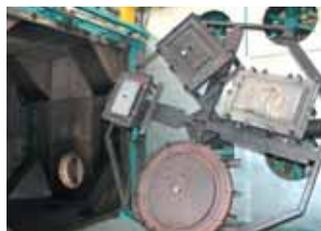
The mould is rotated in a specialised oven.
